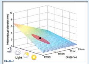
The area of the progressive lens surface that would be in use given the size of the pupil under the specific lighting level and viewing distance combination being modeled is represented in red. The model also takes into account the Rx, add power, and direction of gaze.
