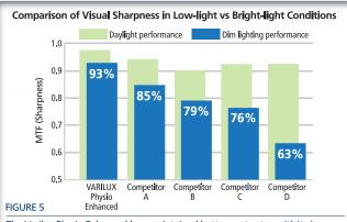
The Varilux Physio Enhanced lens maintained better contrast sensitivity in both low-light and bright-light conditions as indicated by a higher modulation transfer function (MTF). Evaluation based on a –4.00 D lens with +2.00 D add and pupillary diameters of 3 mm (bright light) and 8 mm (dim light).<sup>4</sup>
